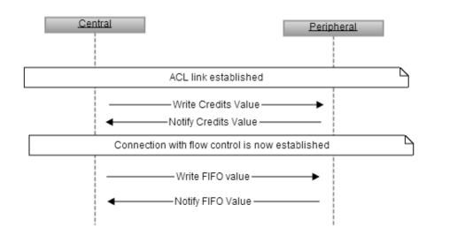
Figure 6: Connection with flow control (bonded)
