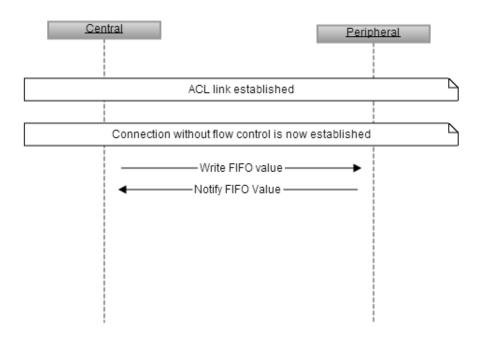
Figure 8: Connection without flow control (bonded)
