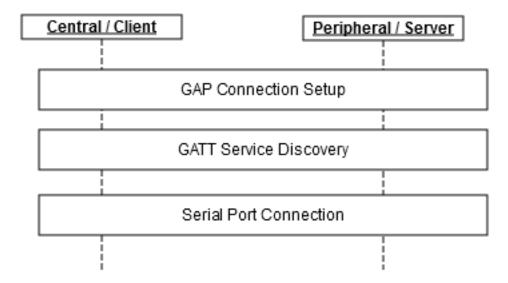
Figure 1: SPS connection setup
