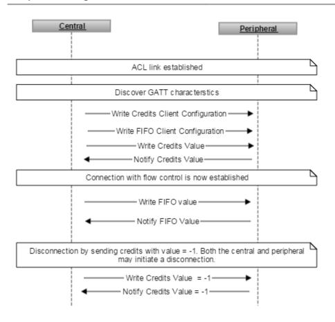
Figure 5: Connection with flow control (non-bonded)
