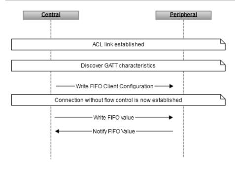
Figure 7: Connection without flow control (non-bonded)
