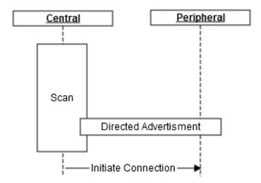
Figure 3: Directed GAP connection setup
